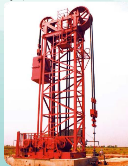
Motor Reversing pumping Unit
